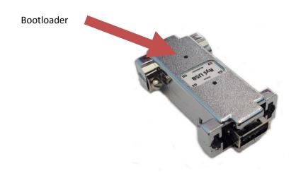
When pressing and holding the **Bootloader** button, one should connect the device via USB cable to the PC running Windows. After being recognized by Windows OS, adapter switches into **Bootloader** mode which is confirmed with continuous pulsation of the **Status** LED.
